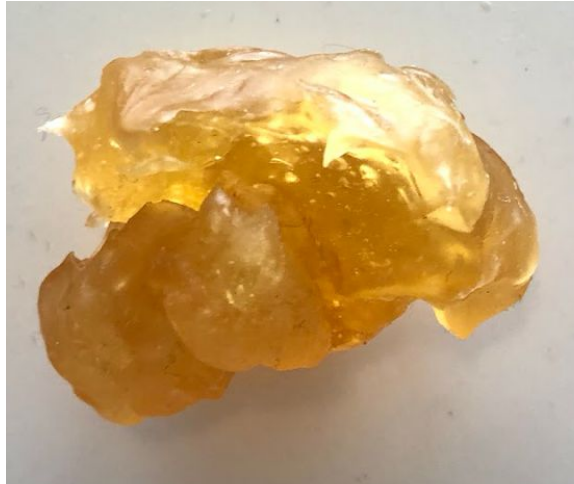
Figure 15: One of the six final I. opaca bioplastics created from the solution. Each of the plastics was allowed to air-dry for two days.
