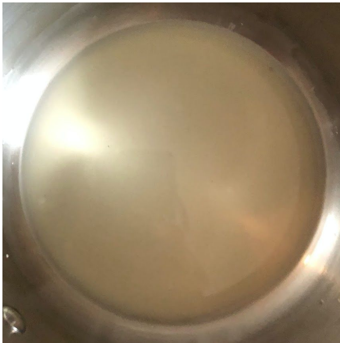
Figure 13: The resulting mixture when the glycerine, acetic acid, distilled water, nutrient-filled I. opaca citric acid solution, and natural polymer were combined.
