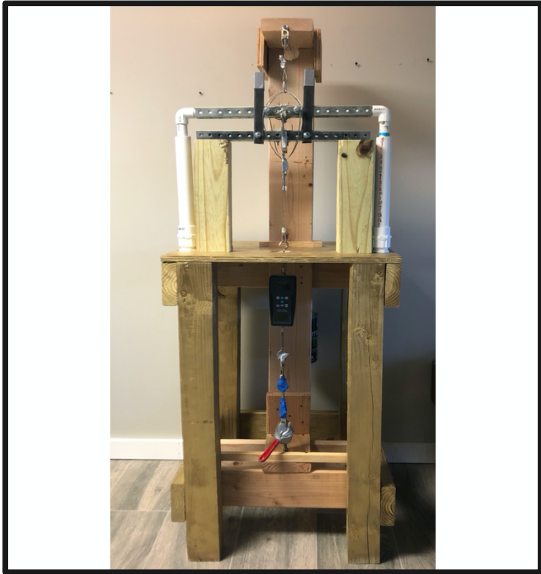
Figure 1: Biomechanical testing device for testing load and displacement
