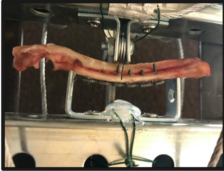
Figure 2—Radius/ulna being tested in 4 point bending
